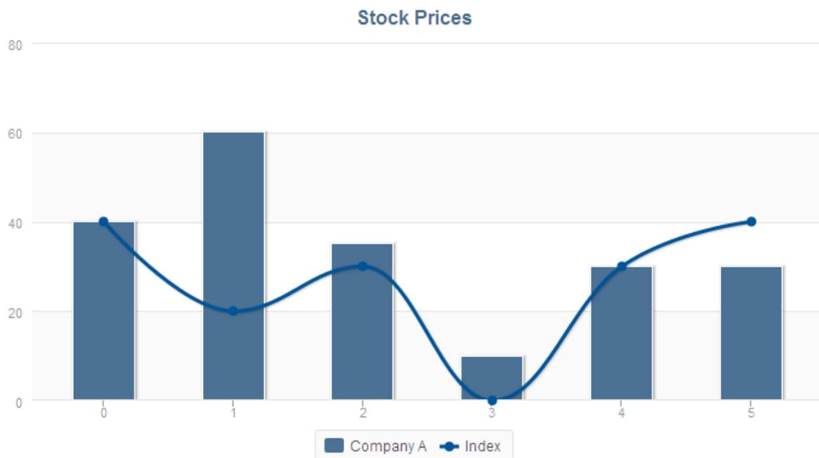
Figure 2.99 Cartesian chart with ListDataSeries (“Company A” and “Index”) and the series definition (further below)
