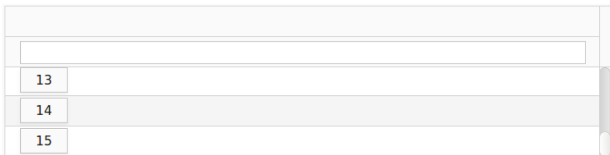
Figure 8.47 Grid with a scroll (the height is set to 3 rows and the data source returns 15 row objects)
