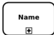
Figure 4.33 Embedded Sub-Process notation
